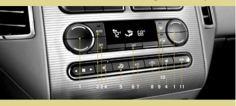
determine fan speed, airflow air temperature. Press location, A/C (on or off) and again to return to interior outside or recirculated air based on your temperature selection. Press again to deactivate.
